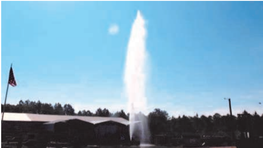
75' Jet of water from a 3" Low Level Pump and a 1" discharge coupling
