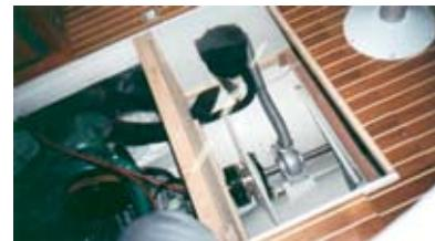
Two different installations of the emergency bilge pump. In each case, the split impeller is installed on the shaft of the vessel in a spaced, non-contacting relationship with the housing.
