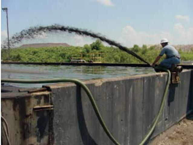
The power behind the double suction pump design is shown here by a 2-in submersible hydraulic unit being used to pump drilling mud solids.
