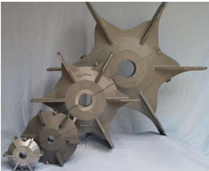
The emergency bilge pump uses a split impeller which comes in a variety of different sizes.
